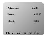
In this menu you can set the date and time and also turn on a continuous time display on the screen.
